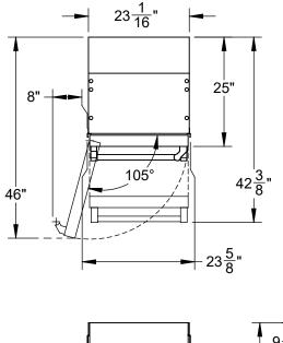
NOTE: A 90° DOOR OPENING IS SUFFICIENT TO ALLOW FULL EXTRACTION OF THE INNER DRAWERS, EVEN IF THE APPLIANCE IS DIRECTLY ADJACENT TO A WALL. HOWEVER IF 105° OPENING IS DESIRED, THEN POSITION APPLIANCE AT 8" DISTANCE SHOWN.
